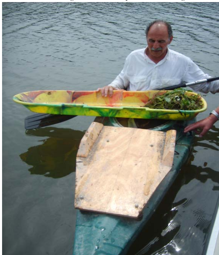
Figure 2-2. Lakeside Restoration’s newly developed water chestnut container system for offloading spoils from a kayak VTDEC
